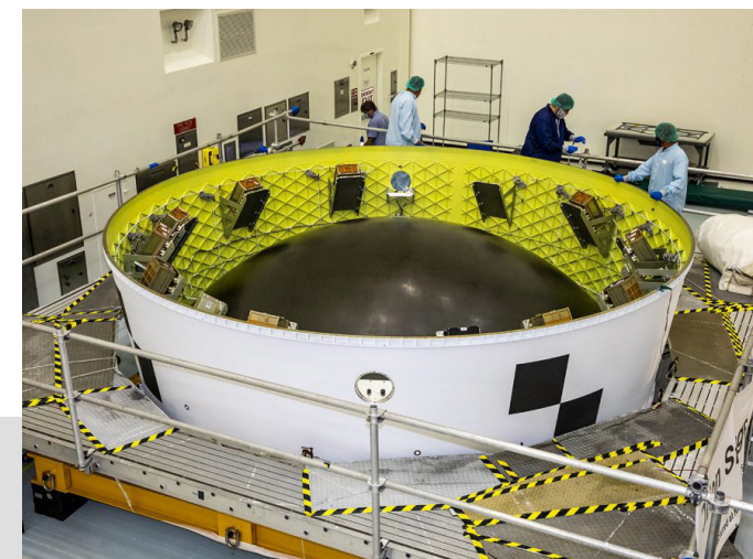
Orion Stage Adapter Ring holding the CubeSats Image/NASA Kennedy Space Center
